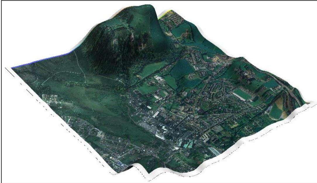
*Killarney High Resolution Ortho Image draped over the 2m Lidar DTM.*
