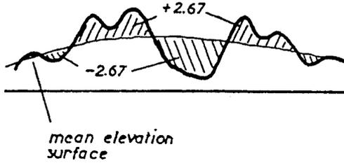
**Fig. 2.** RTM effect principle, from Forsberg (1985). Gravitational effect of the mass surplus and mass deficit of the detailed topography with respect to a mean elevation surface is removed computationally.
