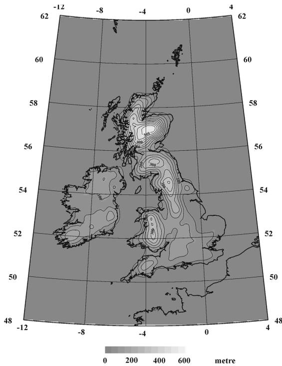
**Fig. 3.** Reference DEM, i.e. a mean elevation surface, obtained from detailed DEMs by filtering, see above, to approximately 66 km spatial resolution.
